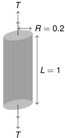
**Figure.** Geometry of torsion of cylinder example.
